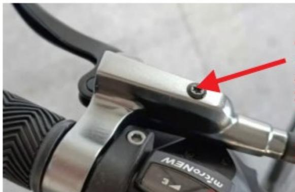
The oil filling hole should be placed at the highest point
